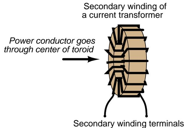
With the power conductor serving as a single-turn<sup>26</sup> winding, the multiple turns of secondary
