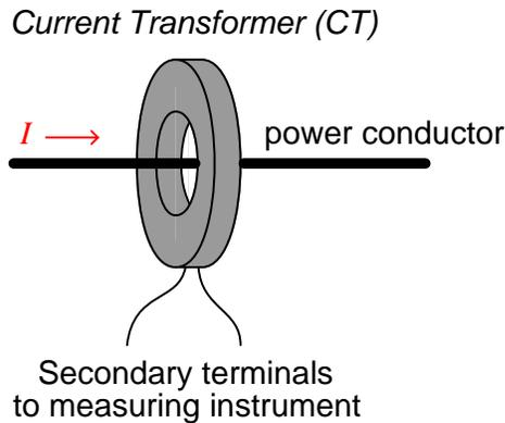
A view of a current transformer’s construction shows the wrapping of the secondary turns around the toroidal magnetic core in such a way that the secondary conductor remains parallel to the primary (power) conductor for good magnetic coupling:
