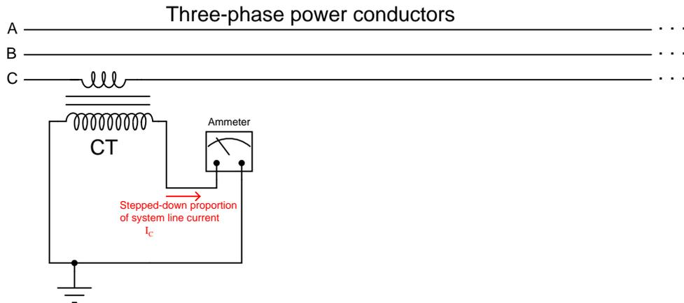
When driving an ammeter – which is essentially a short-circuit (very low resistance) – the CT behaves as a current source to the receiving instrument, sending a current signal to that instrument proportionately representing the power system's line current.
