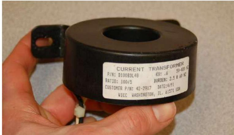
The black and white wire pair exiting this CT carries the 0 to 5 amp AC current signal to any monitoring instrument scaled to that range. That instrument will see  $\frac{1}{20}$  (i.e.  $\frac{5}{100}$ ) of the current flowing through the power conductor.
