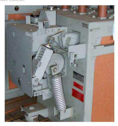
Much like the spring on the hammer of a firearm, the springs inside this Magneblast circuit breaker provide the mechanical driving force for opening and closing the breaker's three electrical power contacts. The act of opening or closing this circuit breaker is analogous to pulling the trigger of a firearm: a small mechanical movement unleashes the stored energy of these springs to do the actual work of rapidly opening and closing the contacts.
