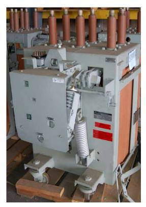
The six "stabs" seen on the top of this breaker unit engage with six sockets connected to the six bus-bar conductors inside the breaker panel (three for the three phases of the line supply, plus three more for the three phases of the load conductors). When this circuit breaker is "racked out," it is dropped down so that these six stabs disengage from the bus-bar connections, making it impossible to energize the load conductors even if the breaker contacts close.
