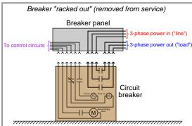
The primary purpose of being able to "rack" a medium voltage breaker into and out of its place in a breaker panel is to facilitate regular maintenance on the circuit breaker mechanism. Unlike the circuit breakers you find in your home, these units may be frequently cycled and will suffer definite wear with each actuation. After a certain number of closing/tripping cycles, the breaker must be removed from service for inspection and testing.
